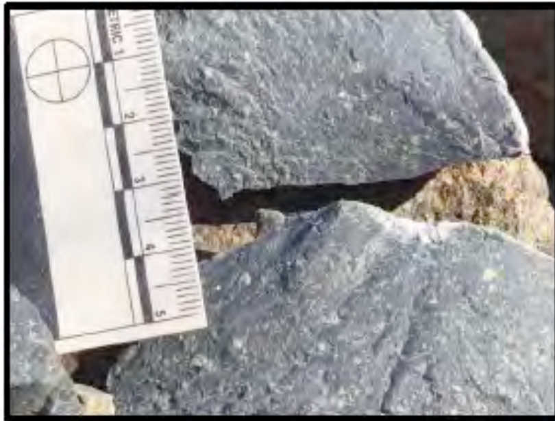
Dacite Hyco volcanic rock sample collected from the Haw River Vicinity near Hwy. 64. This rock type is a viscous lava and forms volcanic domes (cm scale, Bradley, 2021).
